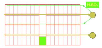
**Figure 1. The layout of the test facility**. Each compartment included 16 pens on fully slatted flooring. Waste pits in two compartments had a 315 mm pull-plug-system installed for removal of waste (control). The other two comprised a waste handling system with sulphuric acid treatment. In this system the treated slurry was pumped through 110 mm pipes from the small storage tank outside the building into the waste pits. Every waste pits in the two compartments were flushed at the same time.
