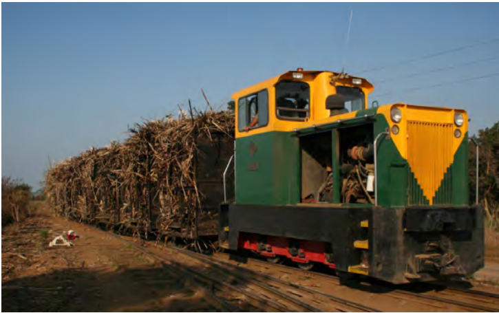
Figure 6. The Narrow gauge locomotive hauling trucks of sugarcane to the Umfolozi mill
